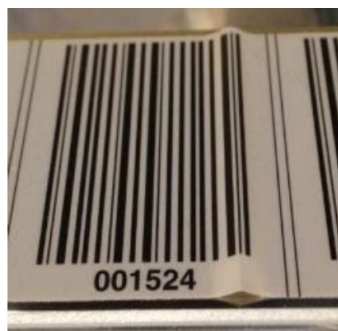
Fig. 36: Cut positioning band at the cutting mark
